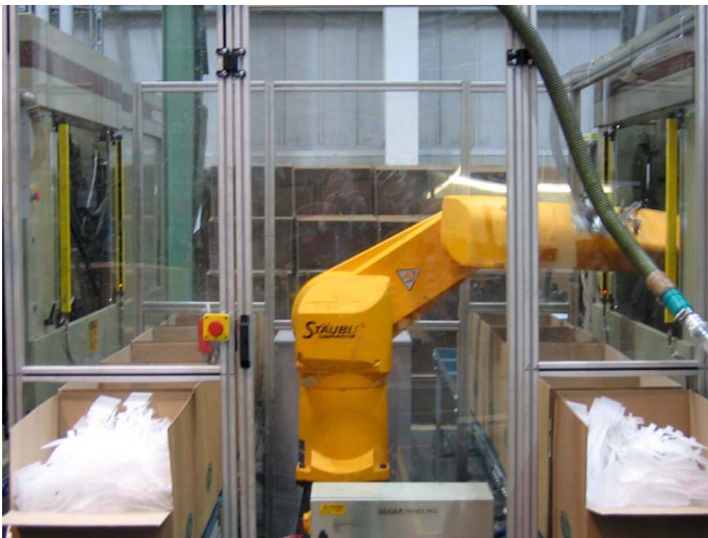
The "Superflag" cell with Stäubli RXplastics 130L robot at ITW Envopak
