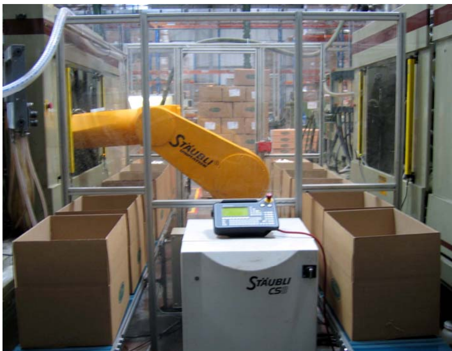
One Stäubli RXplastics 130L robot servicing 2 injection moulders
