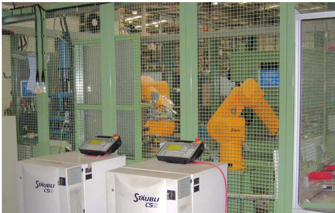
The robotics cell at Simpson Strong-Tie operated by two Stäubli RX90 robots
