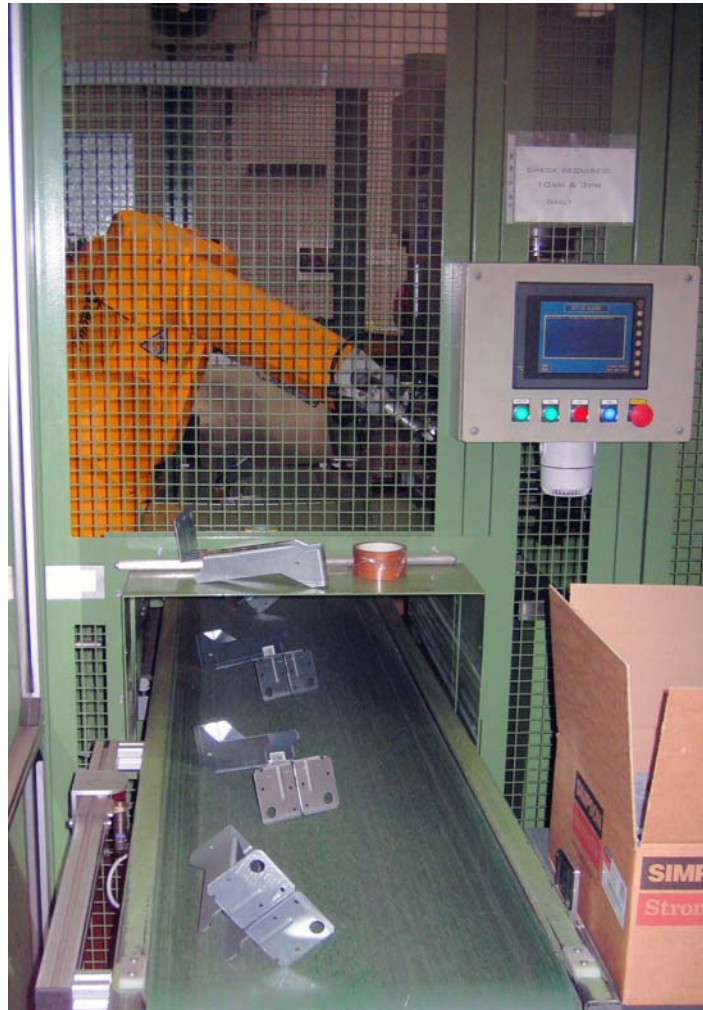
Completed joist hangers leaving the Stäubli Robotics cell
